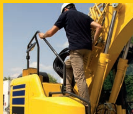
Hand rails and anti-slip plates
