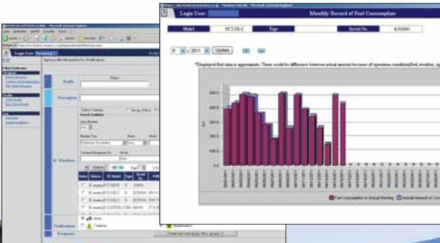
A simple chart shows the machine's fuel consumption and helps you to calculate total costs for a job site and conveniently schedule fuel deliveries.
